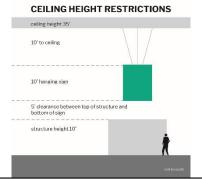
Structure at a max height of 10' Sign at a max height of 10'
