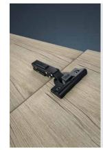
← The T-type Hinge from the **Titus Group** features integrated damping and a performance of 200,000 lifecycles, which is especially important for thicker and heavier cabinet doors where sagging is an issue. The hinge offers wide tolerances and consistent performance on a variety of doors. The three-way, snap-on, intuitive hinge-toplate mounting (top, front and back) makes installation a breeze – especially on tall doors. *Booth S4125* **cabinet.titusplus.com**
